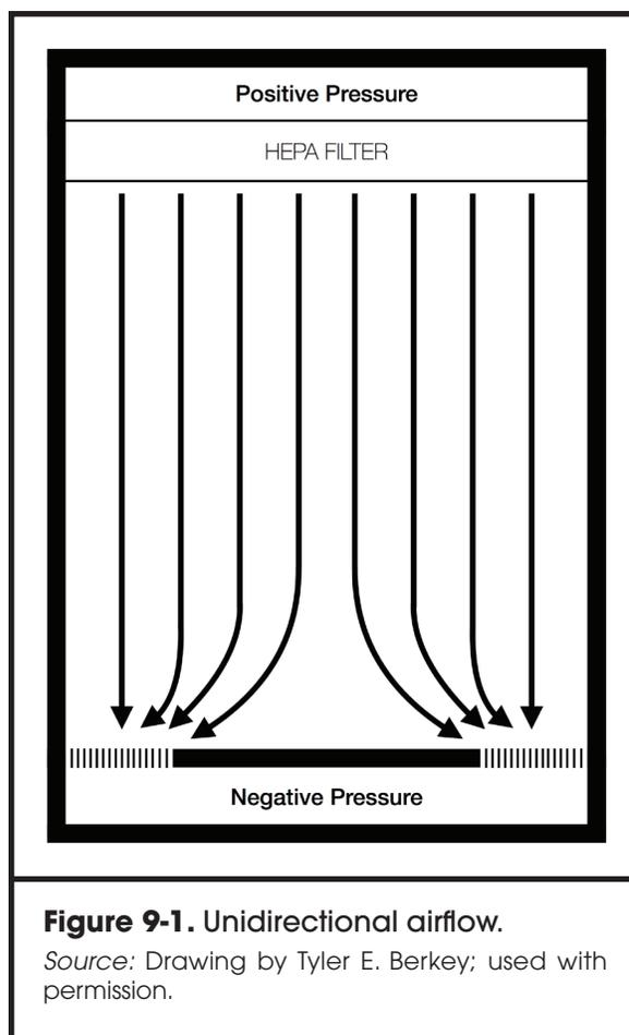
**Figure 9-1.** Unidirectional airflow.
